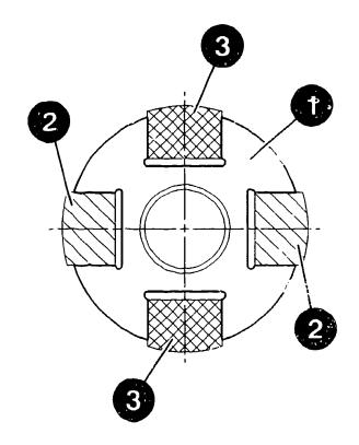
Interchanging of the jaws in the grooves of the yoke results in considerable wear and can cause pump failure.
